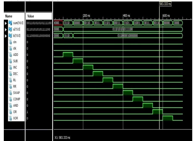
Figure 8: Simulation waveform with 16 bit CALU and 8 bit multiplier.
