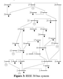
Full Newton power flow method has been performed for simulating the before and after islanding event. Performed power flow study in normal operation data has been compared with [15]. For creating the islanding event, A 40 MW generator and 22 MW load in bus 2 has been isolated from the main grid. The clock has been setup under the bus parameters. For evaluating the microgrid resilience and different distribution a transformer combination has been setup and performed.
