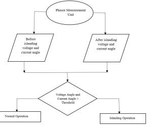
Figure 2:Flow chart to determine islanding operation from phasor measurement unit data
