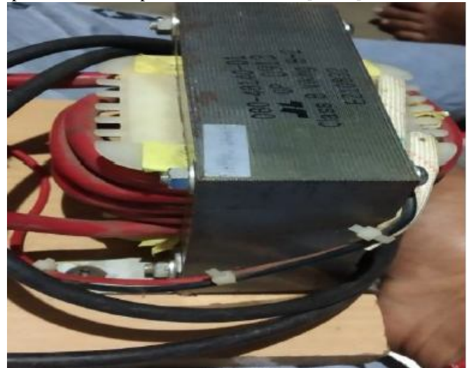
Figure 1: Micro wave oven Transformer
