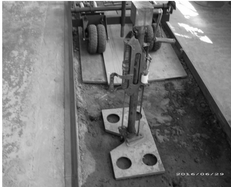
Figure 6: Determination of soil hardness in soil box using Revyakin’s hardness tester
