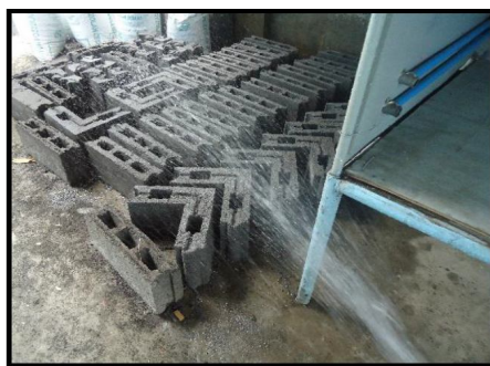
Figure 3: Curing of the mortarless interlocking hollow blocks
