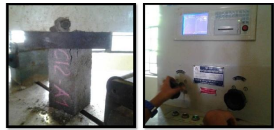
Figure 4: Testing of the mortarless interlocking hollow blocks
