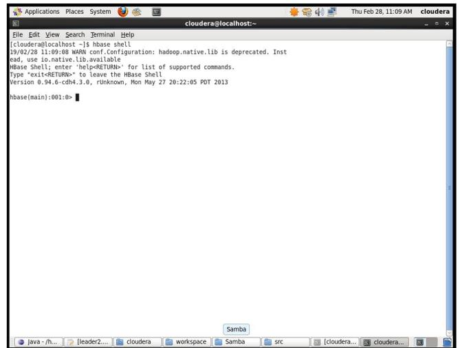
Figure 12: Entering into HBase shell
