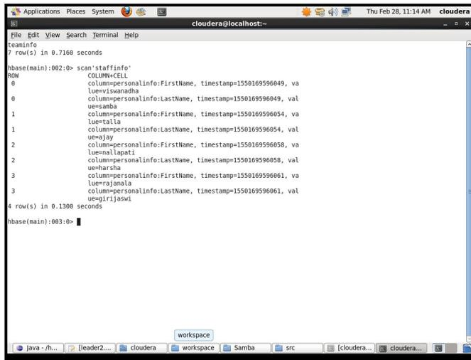
Figure 14: Showing table content in HBase
