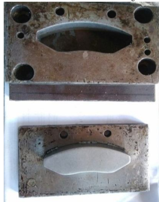
Figure 1: Dies for manufacturing of brake lining
