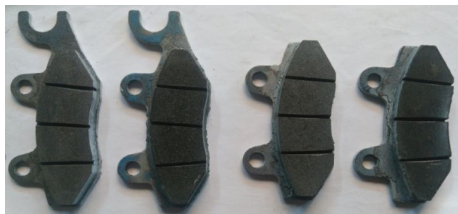
Figure 2: Brake lining made of composite
