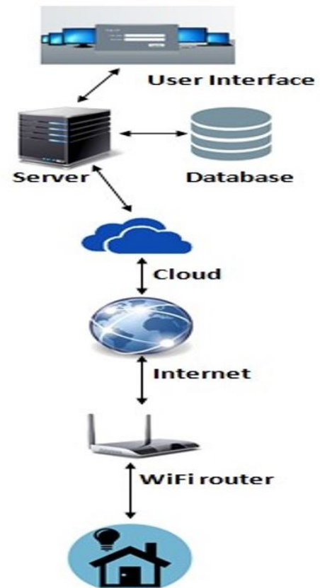
Figure 1: Arrangement Architecture for home automation system.
