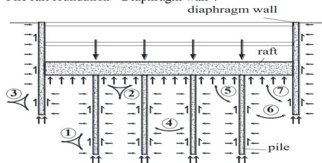
*Noted: 1-Interacted pile and soil; 2- Interacted pift and soil; 3- Interacted DW and soil; 4-Interacted pile and pile; 5-Interacted paft and pile; 6-Interacted DW and pile; 7- Interacted DW and paft.*
