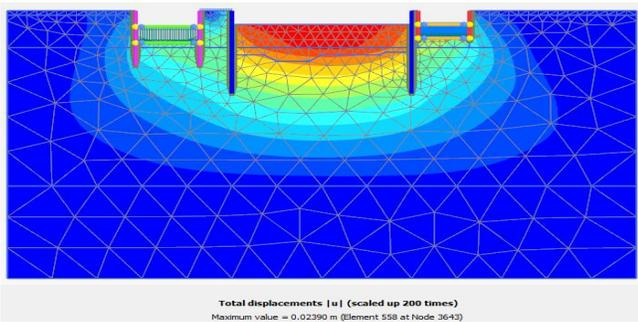
Figure 7. Displacement total
