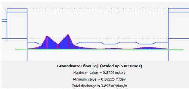
Figure 20. The result of water flowing through the excavation pit's bottom.
