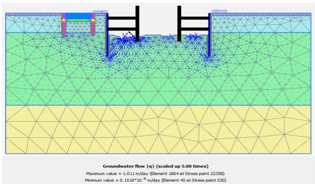
Figure 19. The seepage stress during the excavation stage to the raft foundation's bottom
