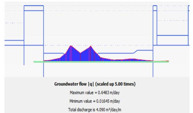
Figure 18. The result of water flowing through the excavation pit's bottom.
