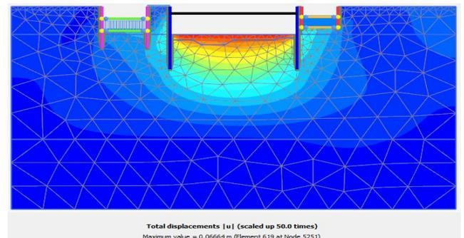
Figure 12. Displacement total
