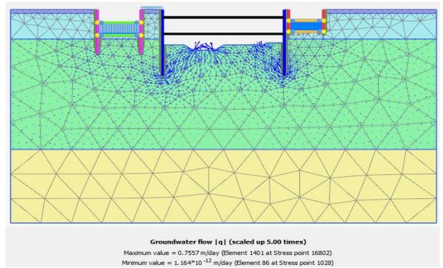
Figure 17. The seepage stress during the excavation stage to the raft foundation's bottom
