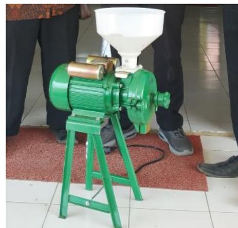
**Figure 7 :** The Prototype of grinding machine
