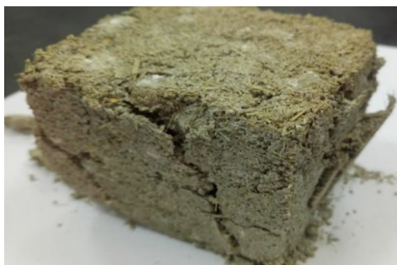
Figure 11 Impact of additives (such as nano-silicon and glass powder) to Cement bricks mixture of ratio (1:4:5) with 3% of rice straw.
