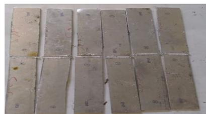
**Figure3(a):** AA5251 & AA6063 Welded Joints
