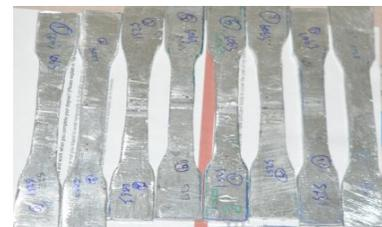
**Figure3(b):** Tensile Specimens as per ASTM Standards
