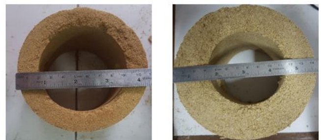
Figure 1: The exothermic sleeve of modulus 1.6 with 2 a thickness of 15mm and 25 mm
