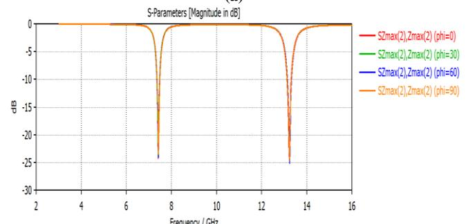
**Figure 2:** Simulated result of reflection coefficient for variations in the angle of polarization under (a)TE mode and (b) TM mode.
