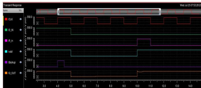
**Figure 4:** Input and Output Signals of the proposed low power NV-MSFF
