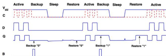
**Figure 2:** Input-Output Signals of the Existing NV-MSFF Signals [12]
