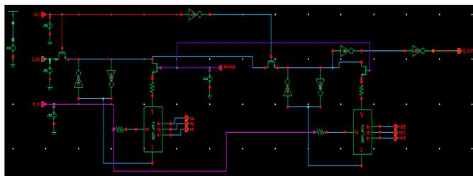
**Figure 3:** Schematic-Diagram of the modified low power NV-MSFF
