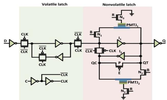
**Figure 1:** NVFF based on three terminal PMTJs based nonvolatile-slave-latch [12]
