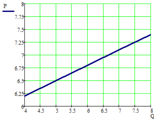
Figure 5: Graphical dependence of the pump power consumption (P, kW) on the pump delivery (Q, m³/h) for a conventional layout.
