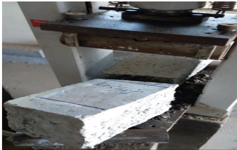
Figure 8 : Setup for Flexure Strength
