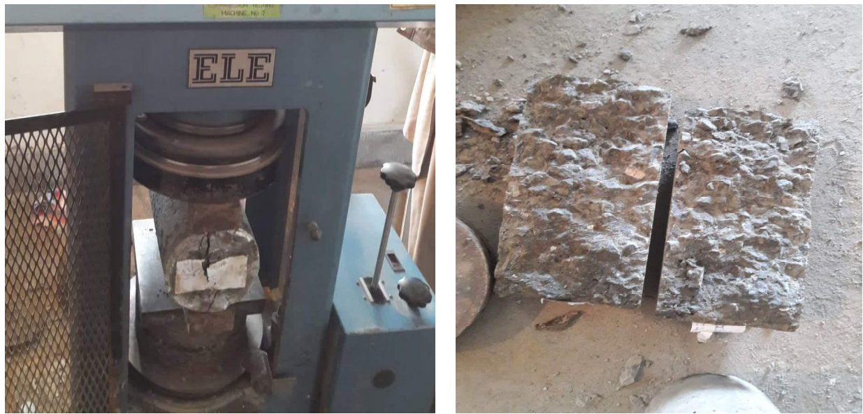
Figure 7 : Setup for Split Tensile Strength
