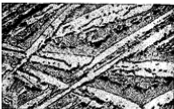
Figure 3: The microstructure of a hypereutectic white cast iron
