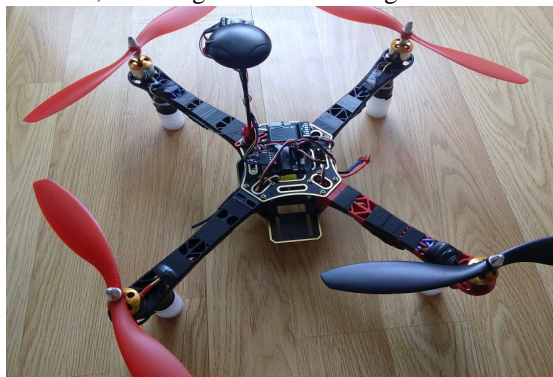
Figure 12: Photo of the experimental copter with the Omnibusf4v3 Controller
