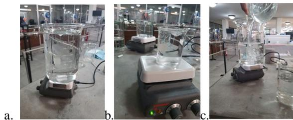
**Figure 1:** The mixture of the chemical components and the distilled water to form 4 liters of formation water. (a) stirrer of distilled water with magnesium chloride salt, (b), several beakers of 1000ml each, where distilled water is mixed with various salts, (c) placing distilled water in a glass of aforementioned to be stirred with the salts. Images captured by the authors.
