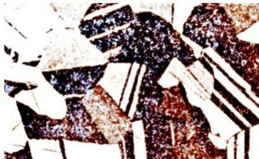
Figure 5: Microstructure of single-phase brass after rolling and firing
