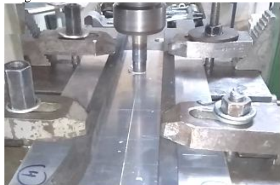
Figure 2: Friction Stir Welding Configuration.
