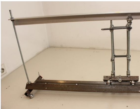
Figure 8 Subassembly of x, y and z axes drive system without lead screw
