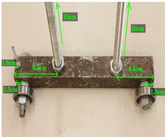
Figure 2 Right subassembly of bar with bearings
