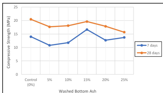
Figure 6: The relationship between the compressive strength and the percentage of washed bottom ash
