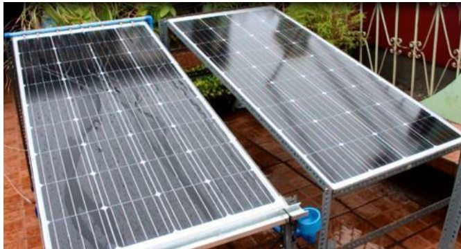
Figure 2: Setup with (left) and without (right) Cooling System
