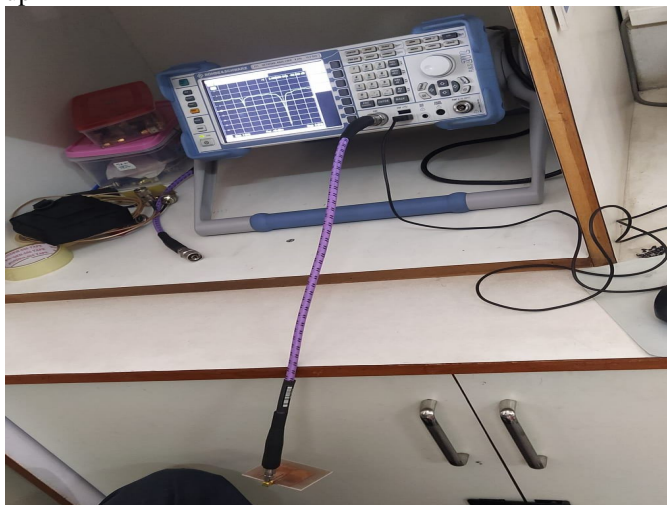
Figure 9. b) : Snapshot of S11 measurement set up by using VNA
