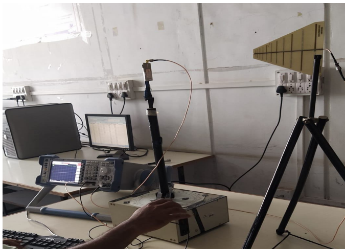
Figure 9. a) : Snapshot of radiation pattern measurement set up
