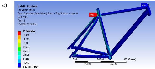
**Figure 3.** Stress distribution on all models (a) Model 1 (b) Model 2 (c) Model 3 (d) Model 4 (e) Model 5
