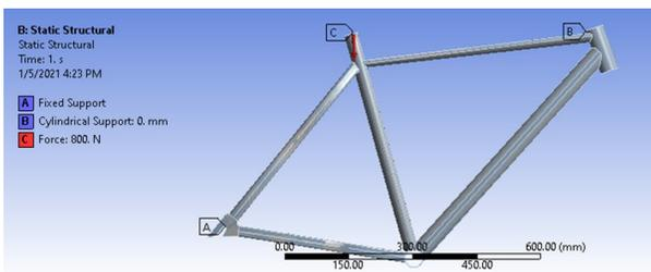
Figure 1. Modeling Frame Tube
