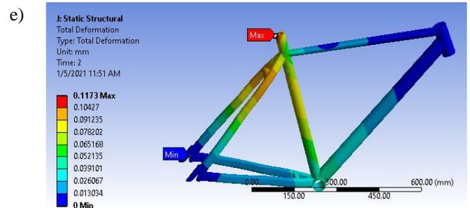
**Figure 4.** Deformation distribution on all models (a) Model 1 (b) Model 2 (c) Model 3 (d) Model 4 (e) Model 5
