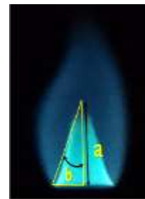
Figure 2: (a). Measurement of the height of the fire, (b). measurement of the angle of fire α
