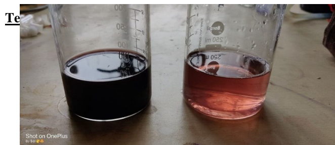
Figure 5.5. Textile Industry dye Effluent degradation before after the experiment using TiO_2 & ZnO
