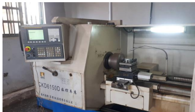
Figure 1: Experimental setup for MQL and dry conditions for the turning test
