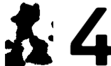
Figure 17. (iii) Left, processed image. Right, character "4". The calculation of the cross-correlation of a matrix (two dimensions) with the third and sixth character is made, which provides sufficient information to make a comparison with characters of similar morphology, as detailed in Table 1.
