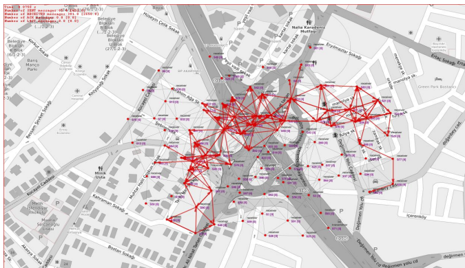
Figure 6. A CupCarbon Simulation Screenshot After a While When Node Communication in Intelligent Traffic Management is Started.
