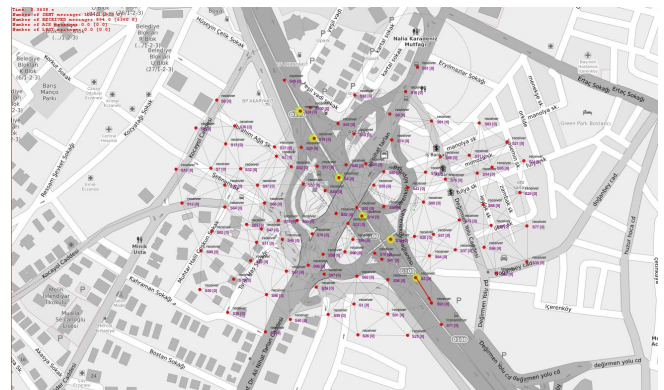
Figure 8. A Screenshot of CupCarbon Simulation Showing Feedback Message Transmission Towards Transmitter Source Node for Node Communication in Intelligent Traffic Management System.
