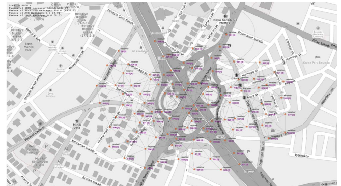
Figure 5. A Screenshot of CupCarbon Simulation at Initial Condition for Node Communication in Intelligent Traffic Management. Total of 100 nodes are assumed to be deployed randomly around Bostancı Bridge in Istanbul
