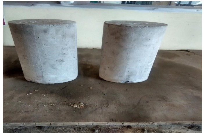
Figure 1: Sample of Specimens (cylinder) for Rebound Hammer Test
