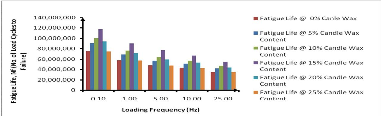
Figure 1: Variation of Fatigue Life with Loading Frequency @ varying Candle Wax Content
