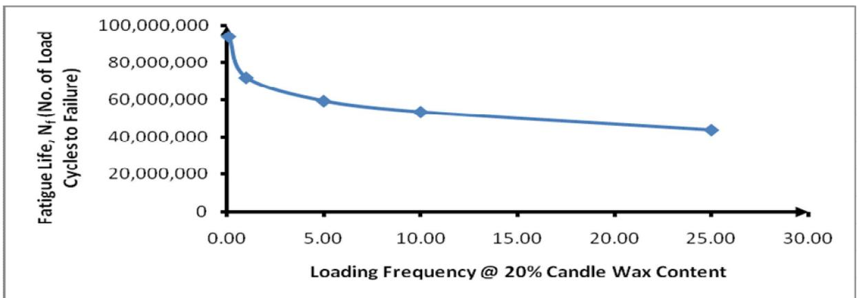
Figure 6: Variation of Fatigue Life with Loading Frequency @ 20% Candle Wax Content
