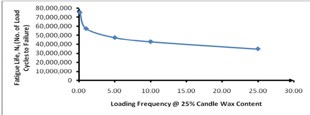
**Figure 7: Variation of Fatigue Life with Loading Frequency @ 25% Candle Wax Content**
