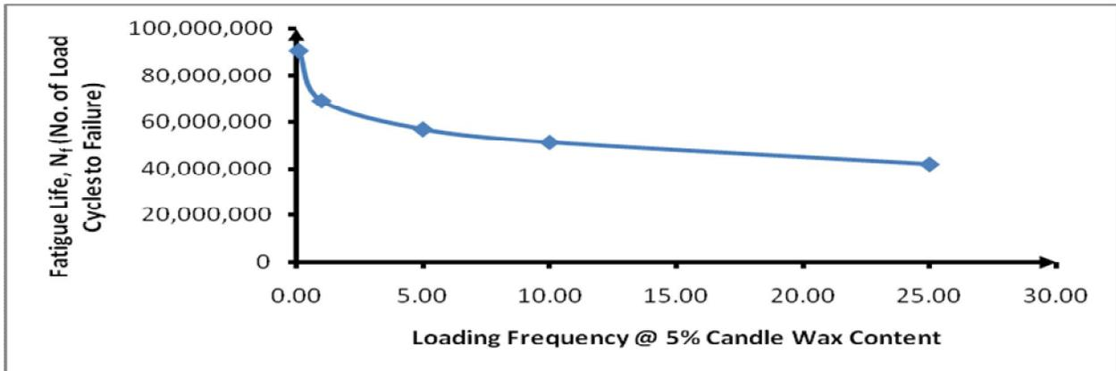
Figure 3: Variation of Fatigue Life with Loading Frequency @ 5% Candle Wax Content
