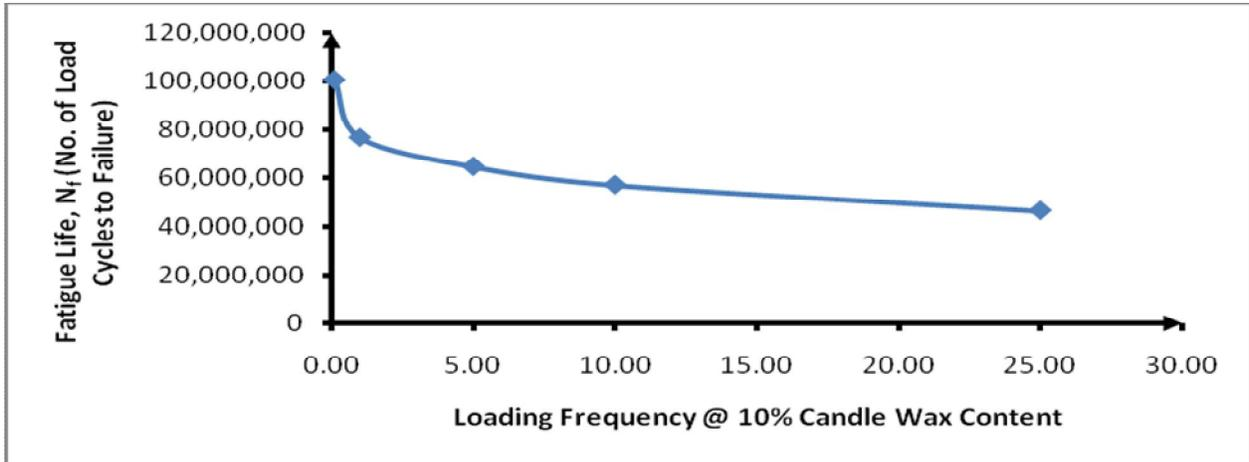
Figure 4: Variation of Fatigue Life with Loading Frequency @ 10% Candle Wax Content
