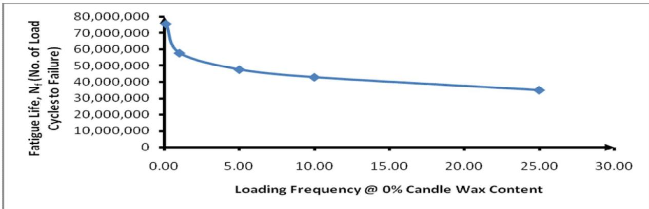
Figure 2: Variation of Fatigue Life with Loading Frequency @ 0% Candle Wax Content
