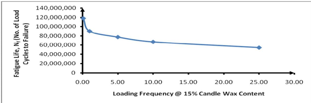
Figure 5: Variation of Fatigue Life with Loading Frequency @ 15% Candle Wax Content
