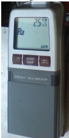
Figure 2: Talysurf (surface roughness measuring machine)
