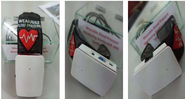
Figure 6: Final design output of the Microcontroller-based Wearable Blood Pressure Monitoring Device with GPS and SMS Feature through Mobile App
