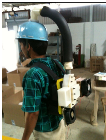
Figure 17: Typical Lab-Trial Photograph by a person using back-pack Thermoelectric Cooling helmet at hot environment.
