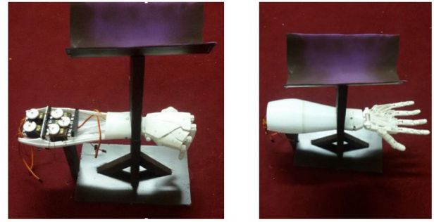
Figure 7: The Humanoid Robotic Hand installed on the stand
