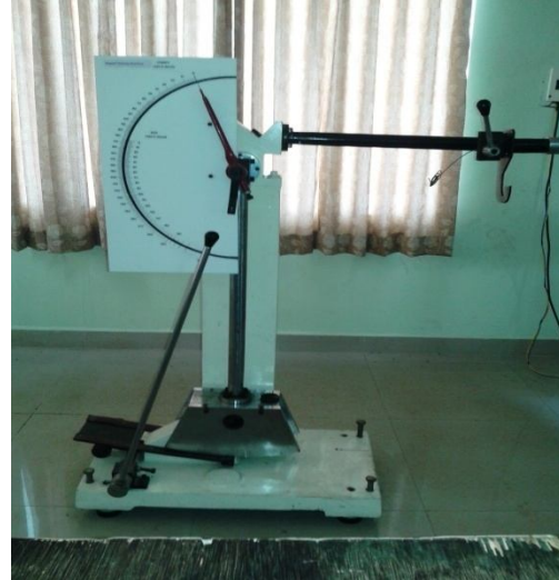
Figure 9. Impact Testing Machine
