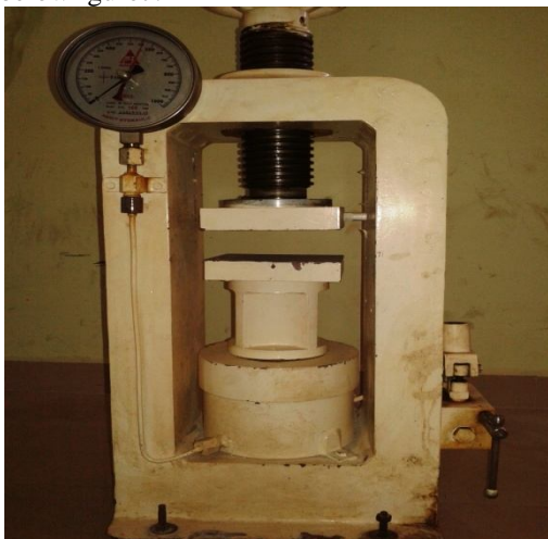
Figure 7. Compression Testing Machine
