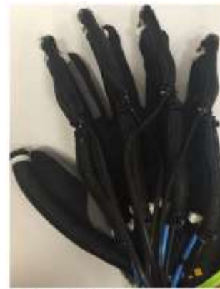
Figure 15: The exoskeleton glove is made by sewing four variable stiffness actuators onto the dorsal side of a traditional worker glove. A solenoid valve controls the muscle filling and venting separately [22].
