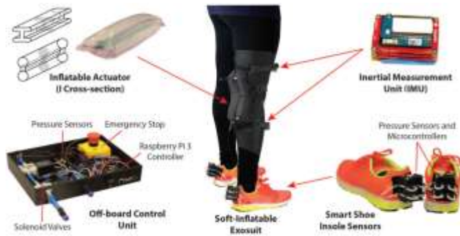
Figure 6: The soft-inflatable exosuit's design [72]
