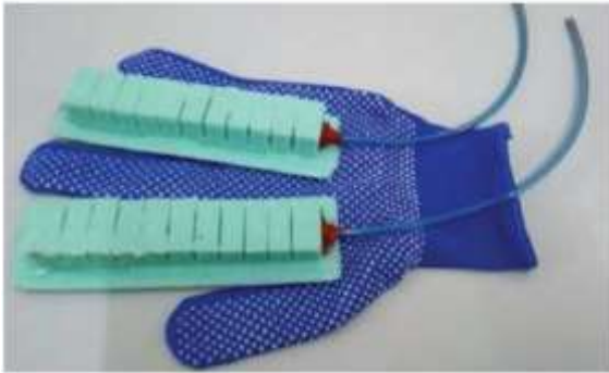
Figure 16: Illustrates the rubber actuators mounted to a nylon glove. The rubber actuator attaches to the top of the nylon glove, and the entrance to the pneumatic tube is entirely closed. RTV silicone was employed as the adhesive agent [97].
