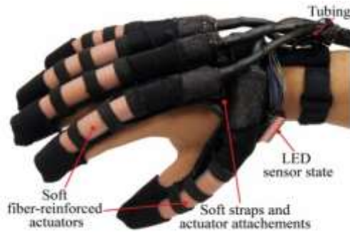
Figure 13: soft robotic glove in which the soft actuators are attached to the dorsal side of the hand providing an open interface to the palm that does not impede the motion [86].
