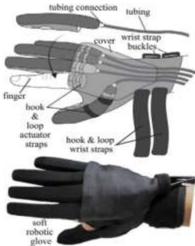
Figure 14: Illustrated the separate textile layers of the glove and the prototype glove [95].
