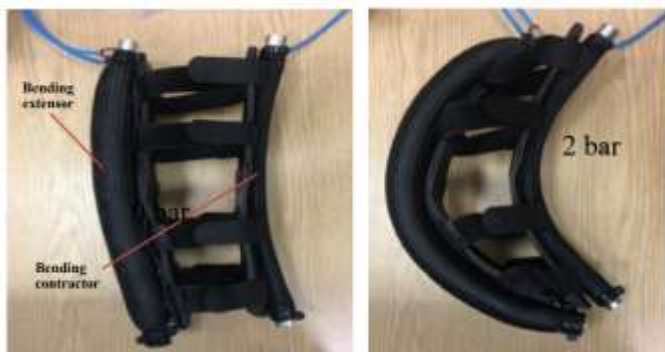
Figure 10: A soft robotic arm for elbow rehabilitation is consisting of soft and bendable parts without separate joints to minimize external structural alignment with the user's arm [79].
