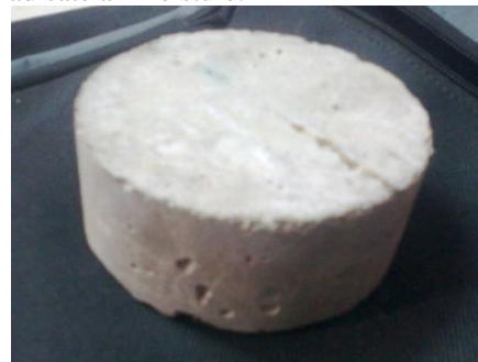
Figure 1: Concrete disc specimen for RCP TEST
