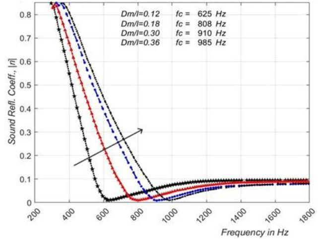
(c) Computed  $|r_i|$  for 4 conductors,  $L=50$ cm and  $D_p=10.62$ cm
