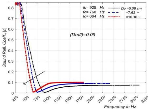
(b) Computed  $|r_i|$  for 3 conductors,  $l=1.0\text{m}$ ,  $D_m=9\text{cm}$
