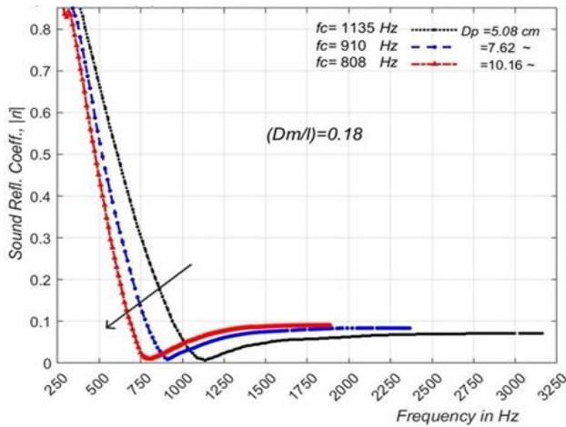
(a) Computed  $|r_i|$  for 3 conductors,  $l=0.5\text{m}$ ,  $D_m=9\text{cm}$
