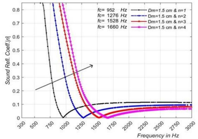
(a) Computed  $|r_i|$  for conductors of  $l=0.5$ m,  $D_p=5.08$ cm, which treated with multi-slit areas of  $D_m=1.5$ cm
