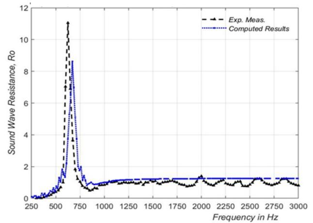
(b) Normalized input sound wave resistance Comp. between measured and computed
