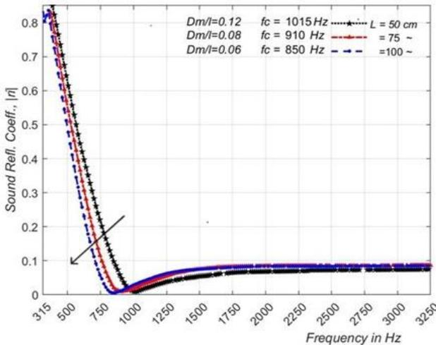
(a) Computed  $|r_i|$  for 3 conductors,  $D_m=6$ cm and  $D_p=5.08$ cm
