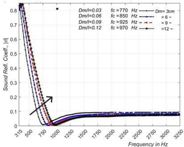
(b) Computed  $|r_i|$  for 4 conductors  $L=100$ cm and  $D_p=5.08$ cm
