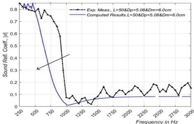
(a) Sound wave refl. Comp. between measured and computed
