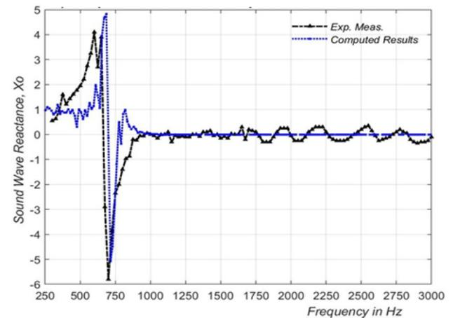
(c) Normalized input sound wave reactance Comp. between measured and computed
