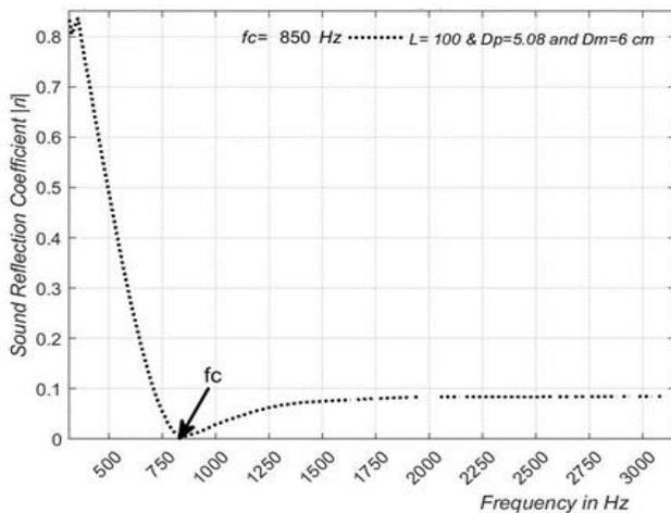
(a) Computed reflection coefficient  $|r_i|$  at the duct inlet
