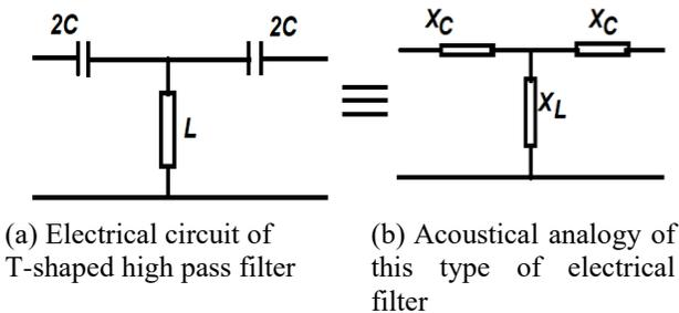
**Figure 2.** Equivalent of acoustic conductor
