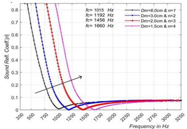
(b) Computed  $|r_i|$  for conductors of  $l=0.5$ m,  $D_p=5.08$ cm, and  $D_m=6$ cm divided into  $n$  slits
