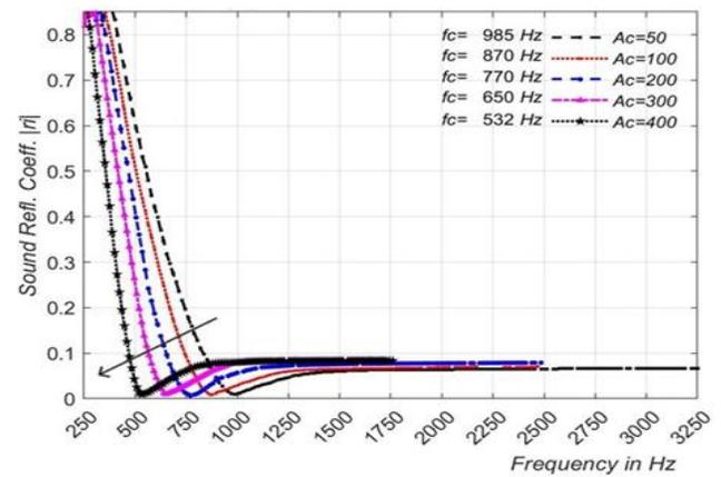
(a) Computed  $|r_i|$  of 5 conductors of different  $A_c$
