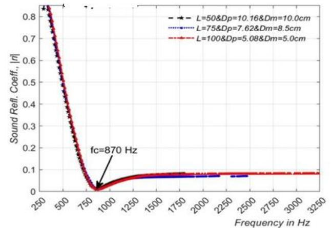
(b) Computed  $|r_i|$  for  $A_c=100 \text{ cm}^2$  of different configurations of  $l, D_p,$  and  $D_m$
