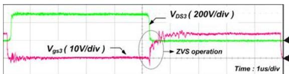
Figure 13. ZVS operation of lagging-leg switches at dual full-bridge mode
