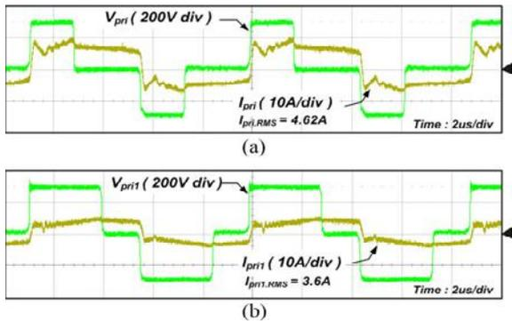
Figure 12. Experimental waveforms of primary voltage and primary current at 20% load condition. (a) V<sub>pri</sub> and I<sub>pri</sub> of the conventional PSFB converter. (b) V<sub>pri1</sub> and I<sub>pri1</sub> of the proposed converter.
