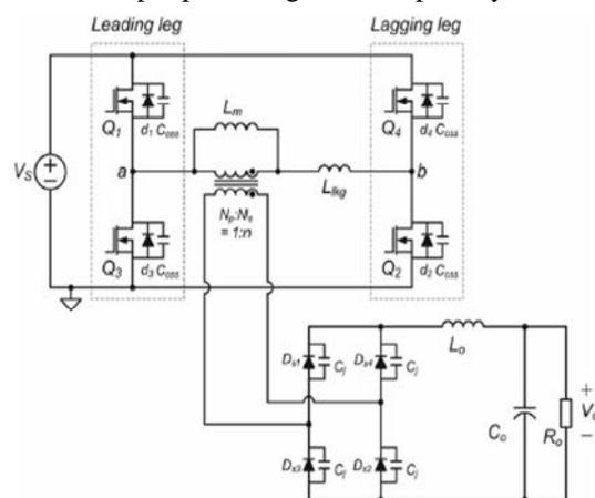
Figure 2. Circuit diagram of the conventional PSFB converter.
