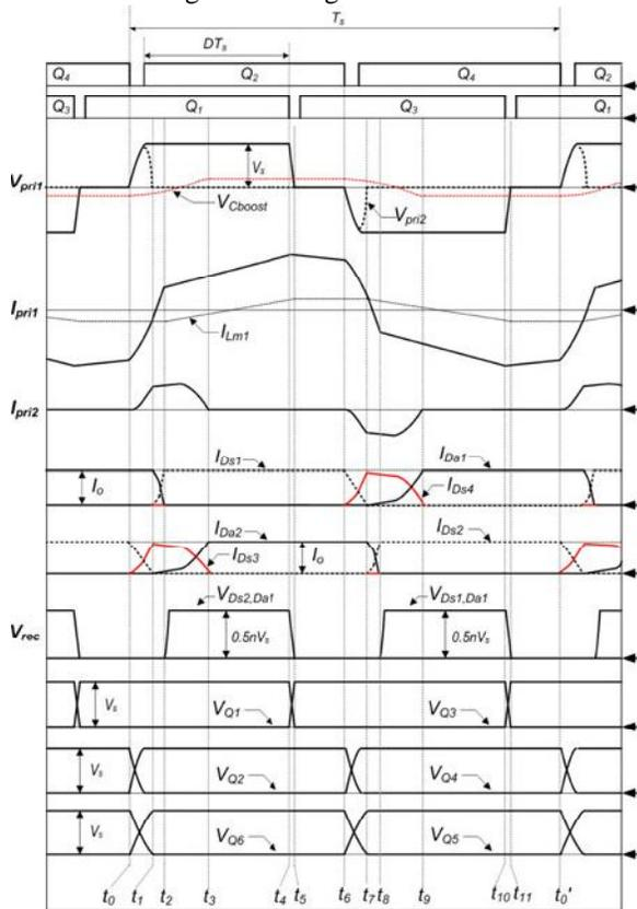
Figure 7. Key waveform at single full-bridge operation.
