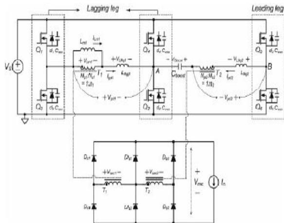
Figure4. Circuit diagram of the proposed PSFB converter at dual full-bridge mode.
