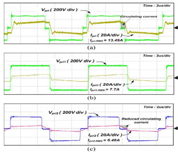
Figure 11. Experimental waveforms of primary voltage and primary current at full load condition. (a)  $V_{pri}$  and  $I_{pri}$  of the conventional PSFB converter. (b)  $V_{pri1}$  and  $I_{pri1}$  of the proposed converter. (c)  $V_{pri2}$  and  $I_{pri2}$  of the proposed converter.
