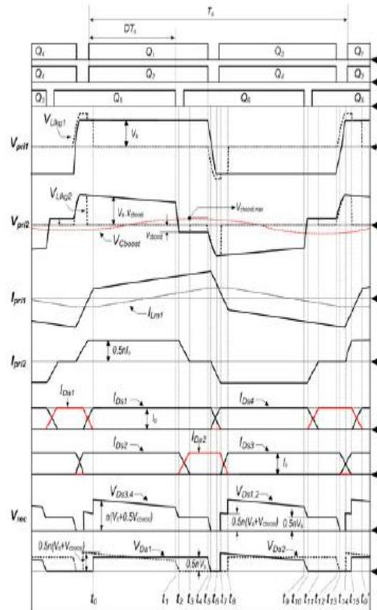
Figure 5. Key waveform at dual-full bridge operation.
