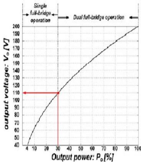
Figure 10. Output voltage profile versus output power.
