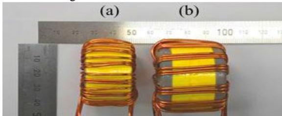
Figure 14. Size comparison of the output inductor. (a) Output inductor of the proposed converter. (b) Output inductor of the conventional PSFB converter.
