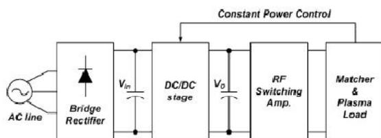
Figure 1. Structure of an RF power generator.
