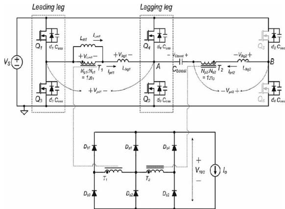
Figure 6. Circuit diagram of the proposed PSFB converter at single full-bridge mode.
