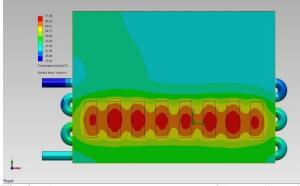
**Fig 4:** FloEFD temperature contours of 25% EGW with 6 LPM flow rate through cold plate.
