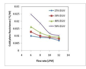
Fig 8: Cold plate Thermal resistance versus flow rate (Simulation)
