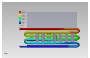
**Fig 5:** FloEFD pressure drop of 50% EGW with 12 LPM flow rate through cold plate.
