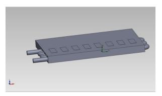
Fig 1: Isometric view of cold plate with heat sources
