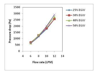
Fig 7: Pressure drop versus flow rate (Simulation)
