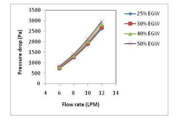
Fig 3: Pressure drop versus flow rate (Theoretical)
