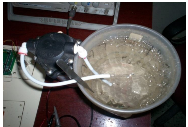
Fig.16. Water pump load
