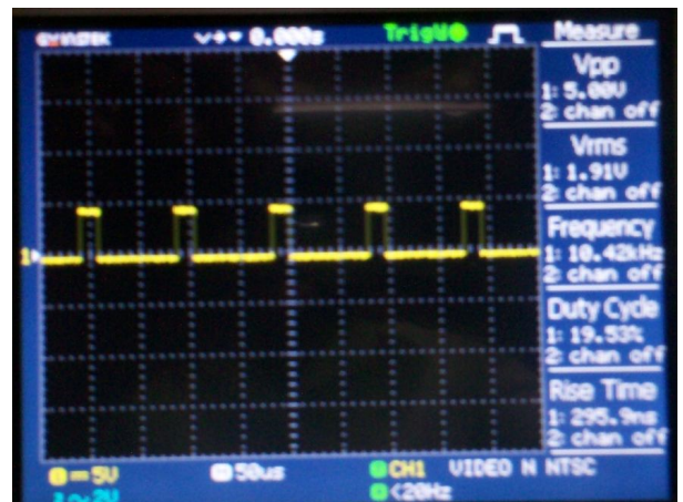
Fig.17. Pulse generation for 20% duty cycle
