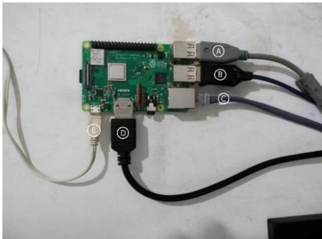
Figure 2a. Connecting the Peripherals of RPi
