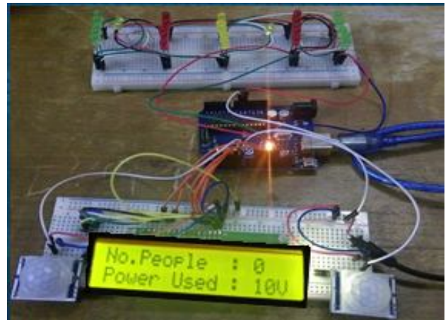
Figure 8: System Testing – No people detected with lower value of volt.
