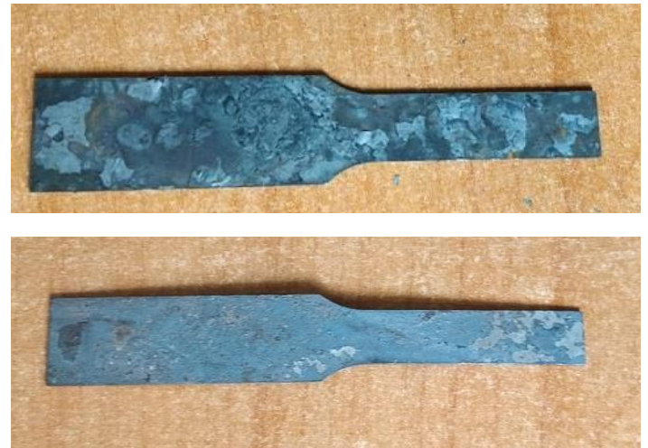
Figure 2: Water Quenched Sample and Air Cooled Sample
