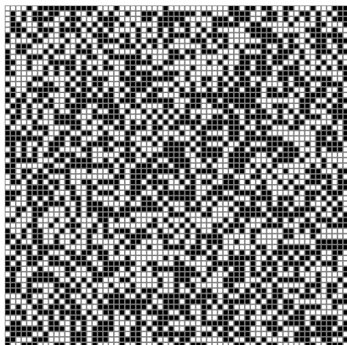
Figure 7: The model of the proposed AR marker is a container containing the obtained permuted image, which is shown in Fig. 6; each cell is 8 \times 8 pixels in size, including a 1-pixel frame
