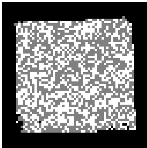
Figure 12: The pixels of the bit container (Fig. 11) are inserted with the correct off set into the N \times N matrix, the undefined values are shown in black, the offset values are by a separate algorithm proposed by the author and will be described in a separate article
