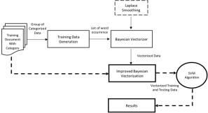
dimensionality and to improve the accuracy of the classification. Figure 1 shows the improved model applied for text vectorization.
